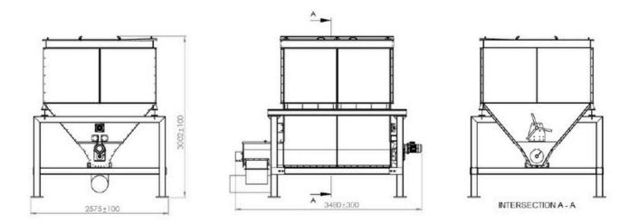
Feeding and emptying of the UBD tanks can be organized in various ways: with the use of a rotary valve, a screw or chain conveyor or pneumatic transport.
